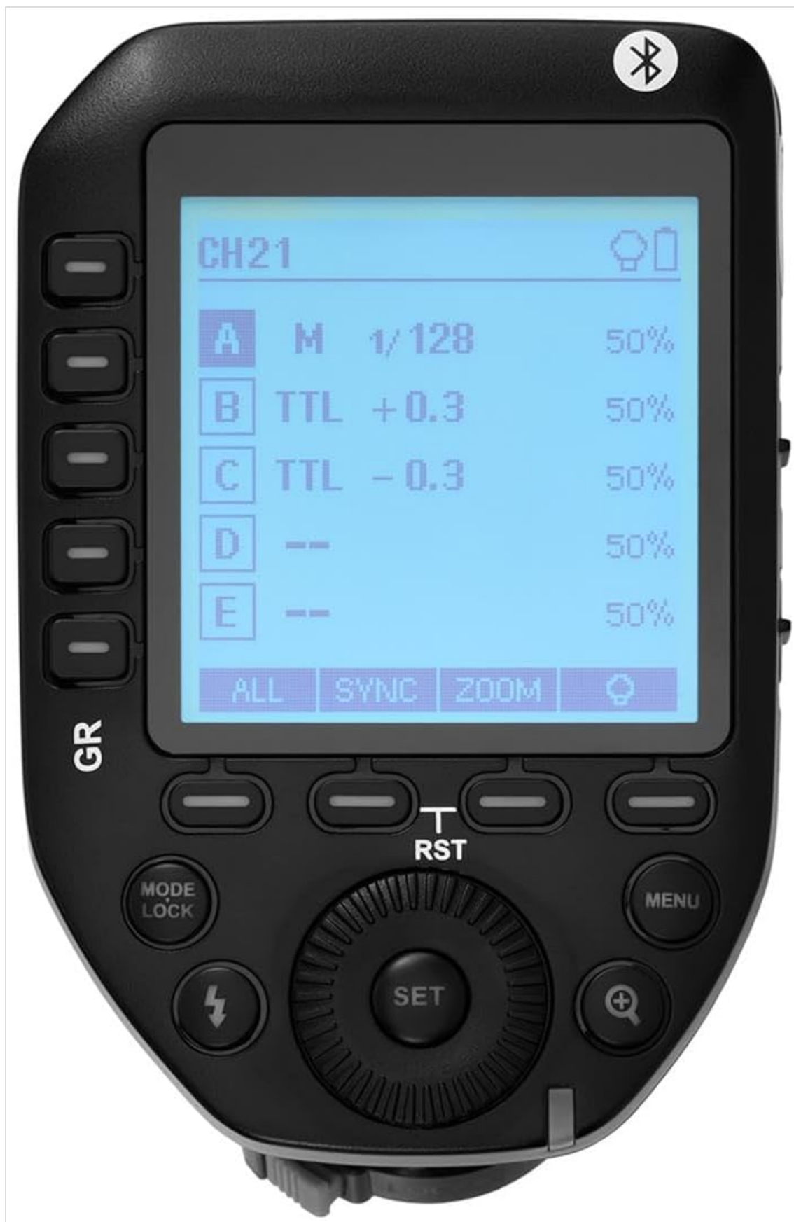
Figure 3.1: Top view of the Flashpoint R2 XPro II, highlighting the large dot matrix LCD display and various control buttons including Group (GR), Mode/Lock, Set, Menu, and Zoom.
