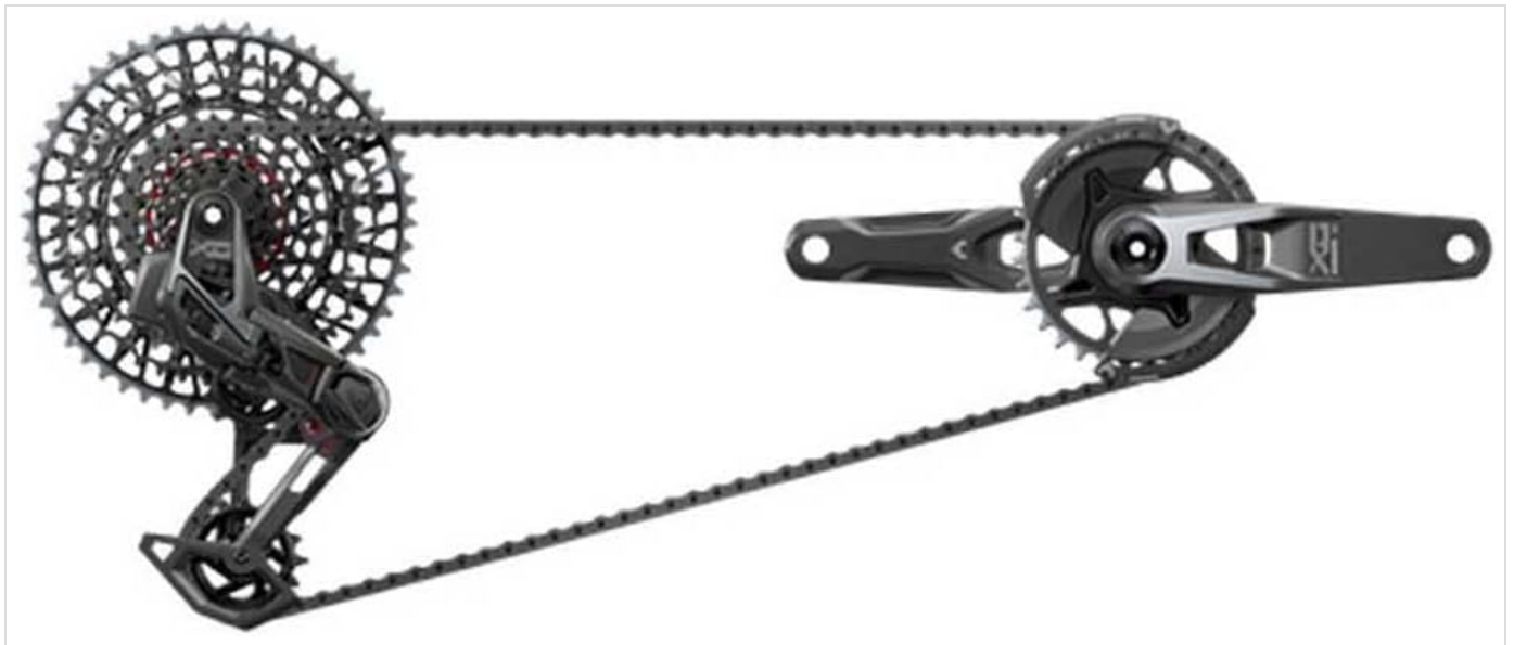
Image 1.1: Overview of the SRAM X0 Eagle AXS Transmission Groupset, showing the rear derailleur, cassette, chain, and crankset.
