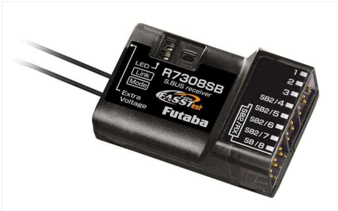
Figure 1: Front view of the Futaba R7308SB receiver, showing the model number, LED indicators, and port labels.
