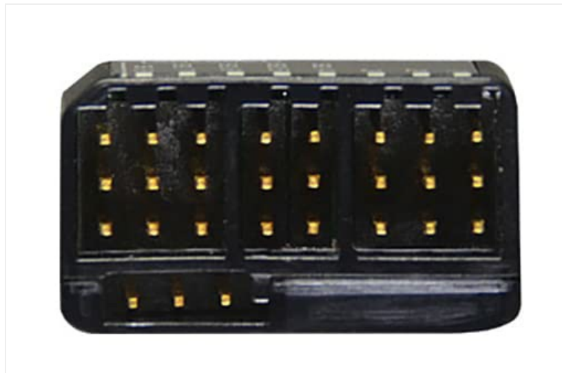
Figure 3: Detailed view of the receiver's output ports, including S.BUS2 and conventional channels 1-8.
