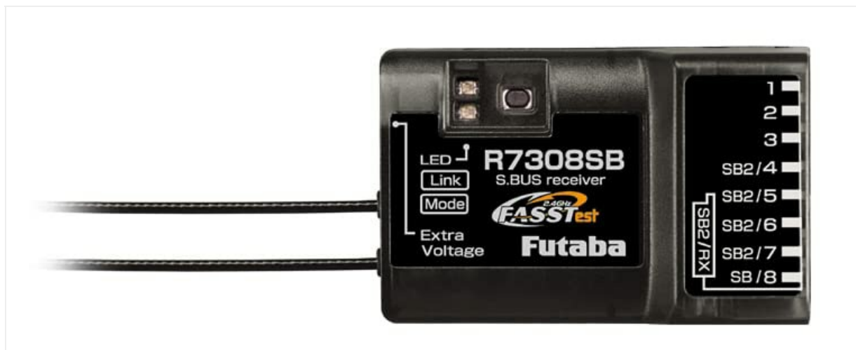
Figure 4: Top view of the R7308SB, highlighting the LED indicator and the Link/Mode button used during the binding process.
