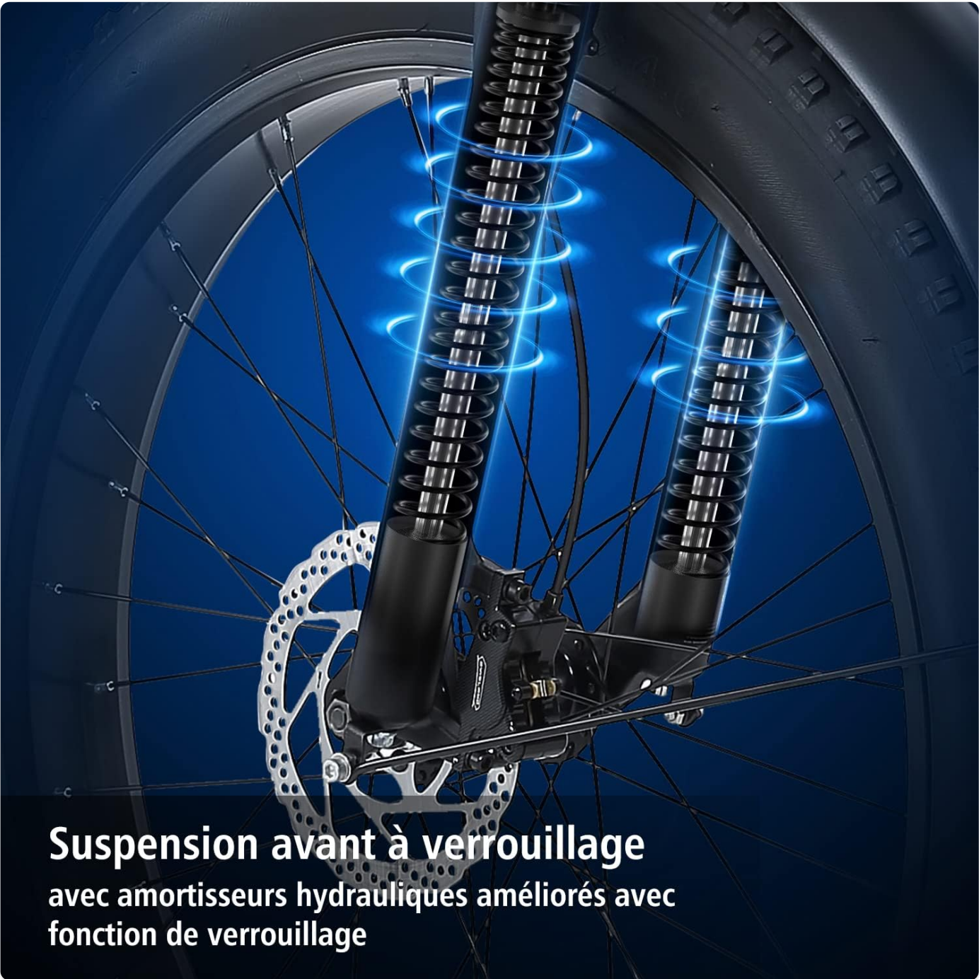
Image: An illustration of the front suspension system of the BURCHDA R5pro, indicating its shock-absorbing capabilities for a smoother ride.
