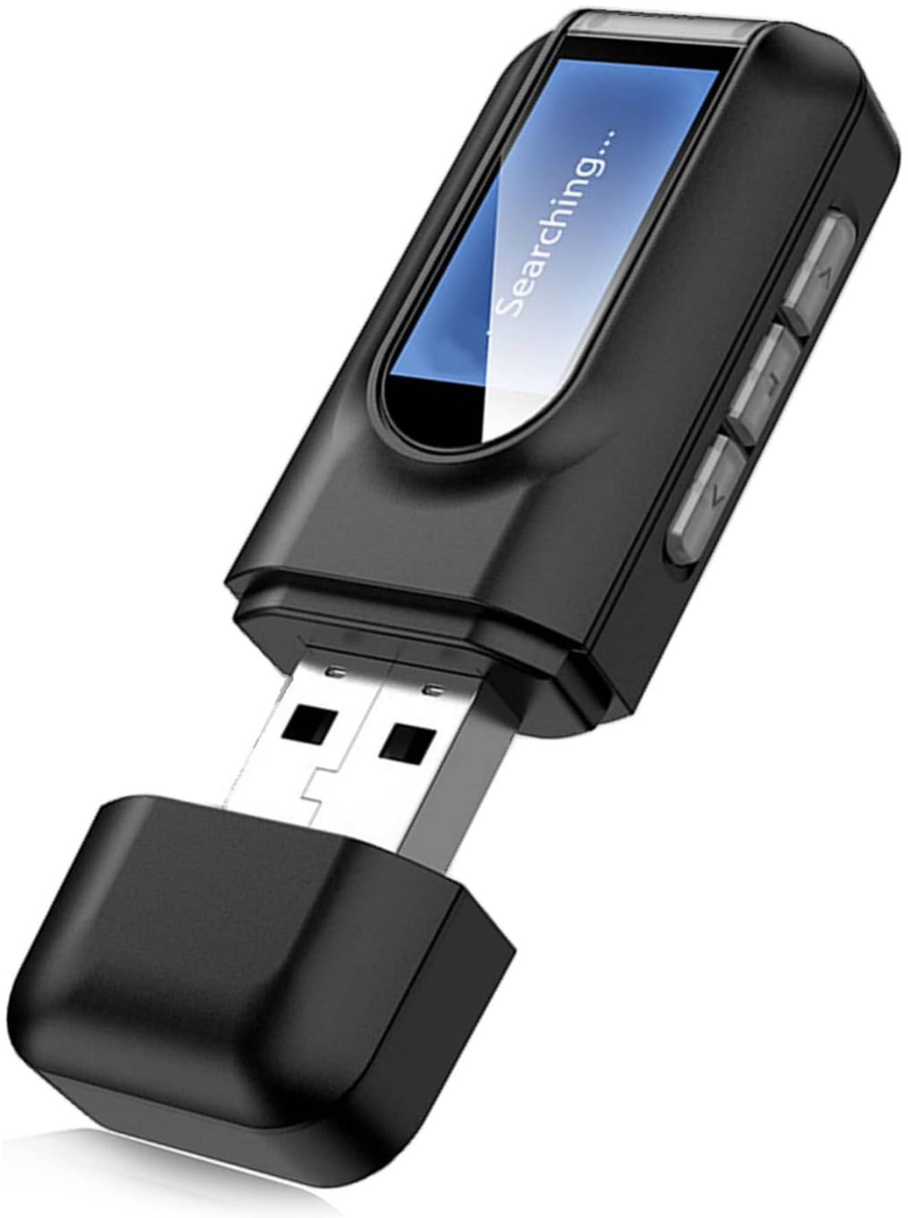
Image 1.1: The Yoidesu Bluetooth 5.0 Transmitter Receiver, showcasing its compact design and LCD screen.
