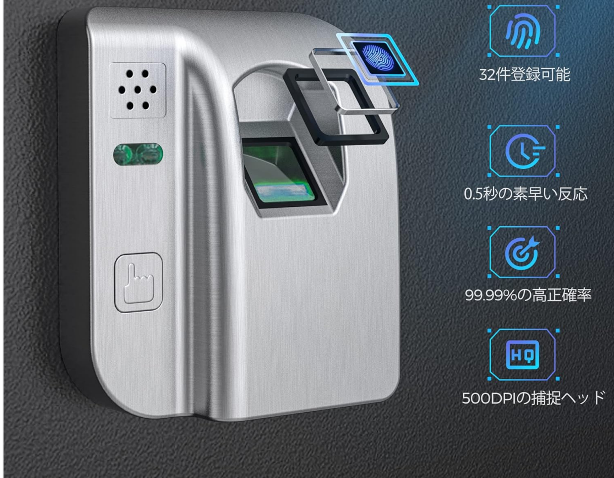
Figure 3.1: Fingerprint Authentication Module. This image shows the high-precision semiconductor sensor capable of registering up to 32 fingerprints, with a 0.5-second response time and 99.99% accuracy.
