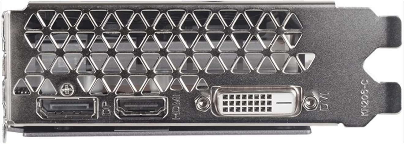
Image: Rear view of the graphics card, detailing the DisplayPort, HDMI, and DVI output connectors.
