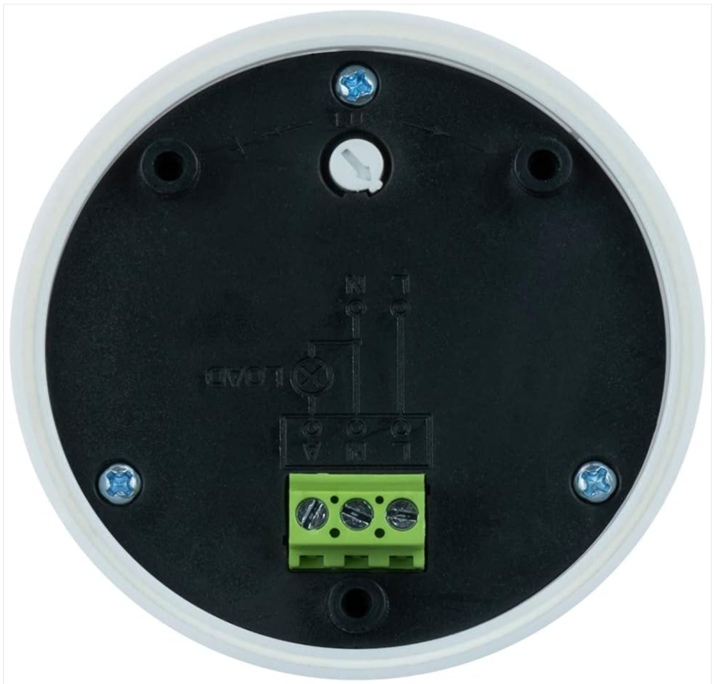
Figure 3: Internal view of the sensor base showing the screw terminals and wiring diagram. Connect Live (L), Neutral (N), and Load (L') as indicated.
