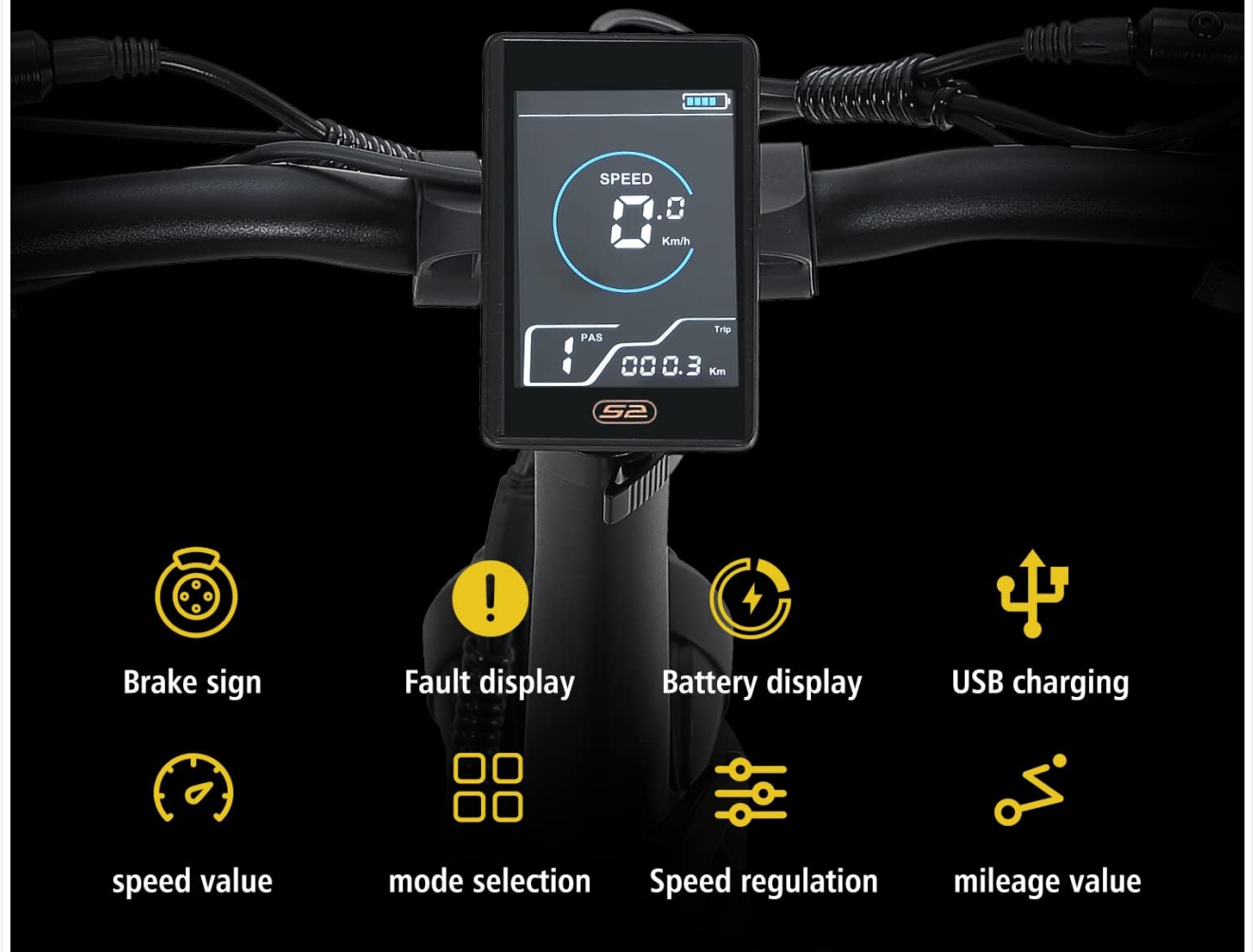
Figure 3.5: The intelligent LCD display provides essential riding information at a glance, including speed, battery, and mode selection.
