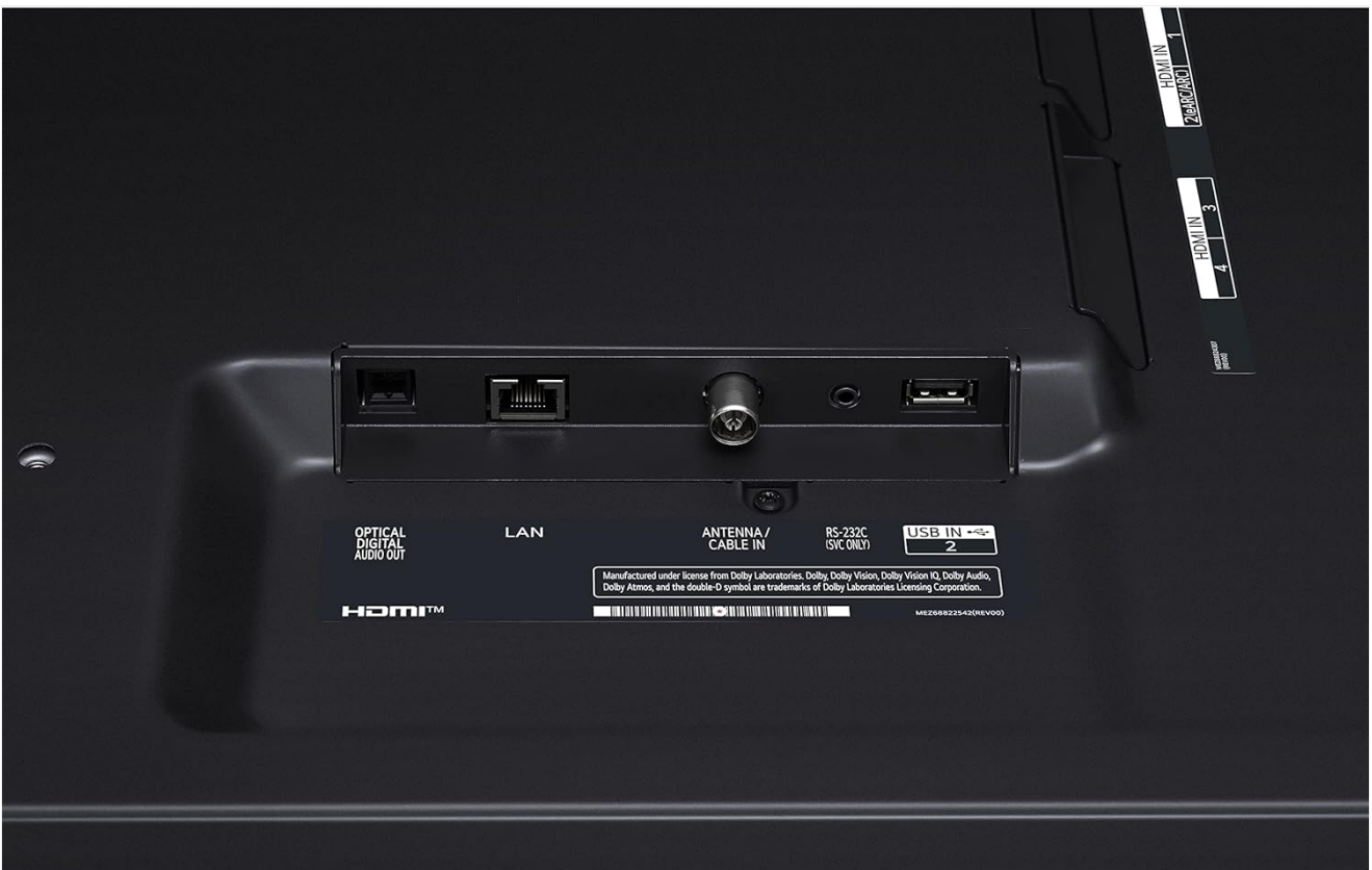
Figure 2.3: Close-up view of the rear connectivity options, including Optical Digital Audio Out, LAN, Antenna/Cable, and USB ports.
