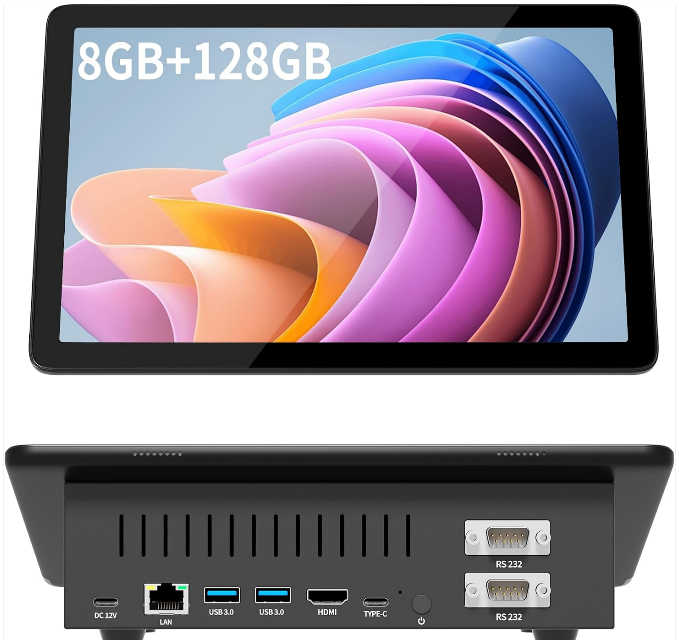
Image: Front view of the HIGOLEPC F10 PRO showing the 10.1-inch touchscreen, and rear view detailing the various input/output ports.
