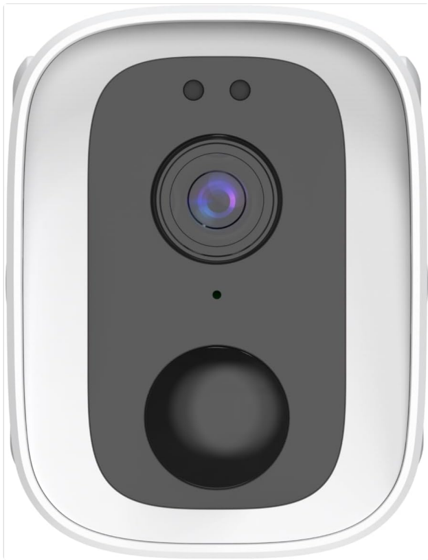
Front Panel: A direct front view of the camera, detailing the central lens, the light sensor, and the infrared LEDs for night vision. The lower circular element is likely the microphone or a motion sensor.
