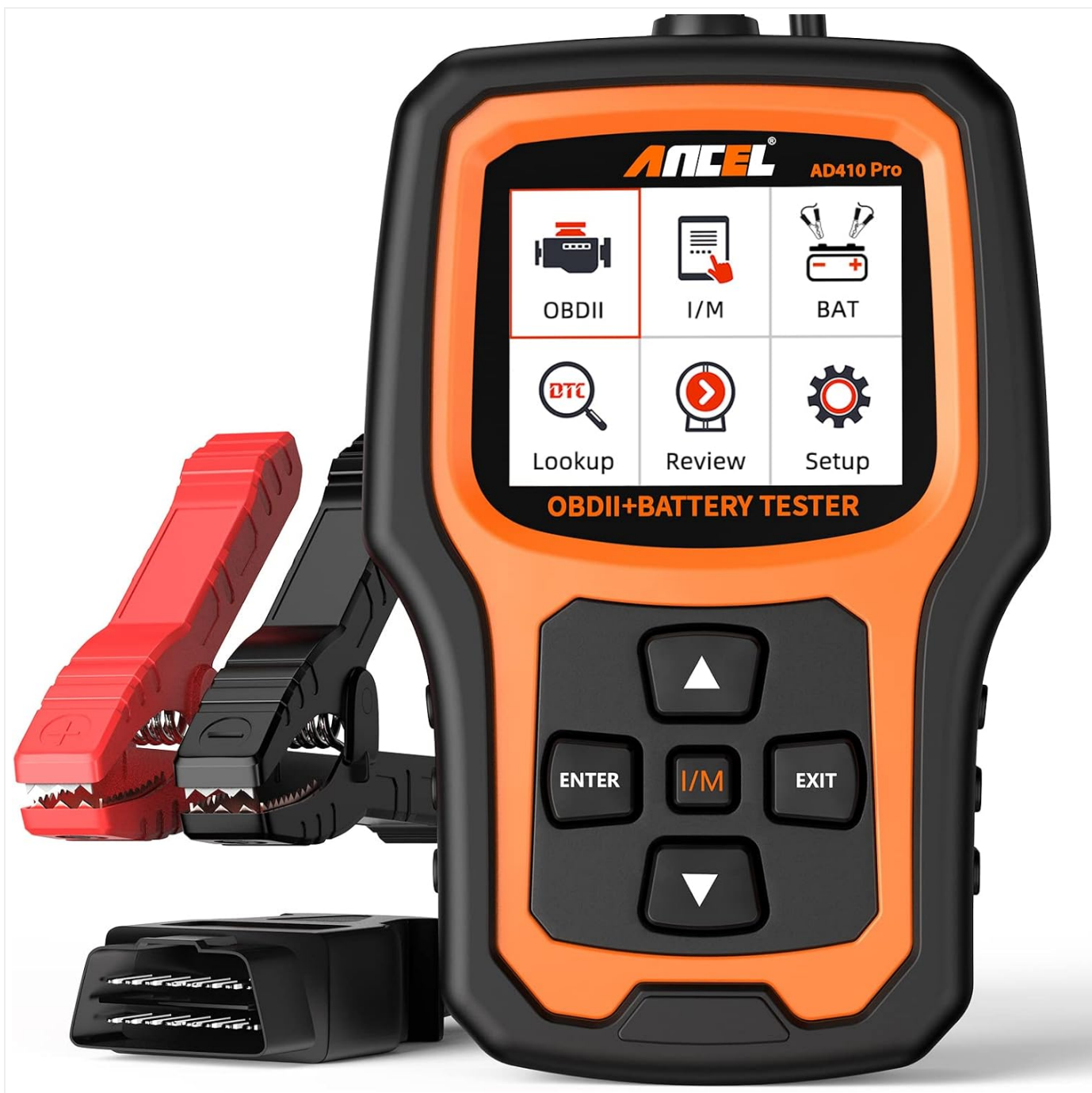
Image: Close-up of the ANCEL AD410 PRO's main screen, showing options for OBDII, I/M, BAT (Battery), Lookup, Review, and Setup.
