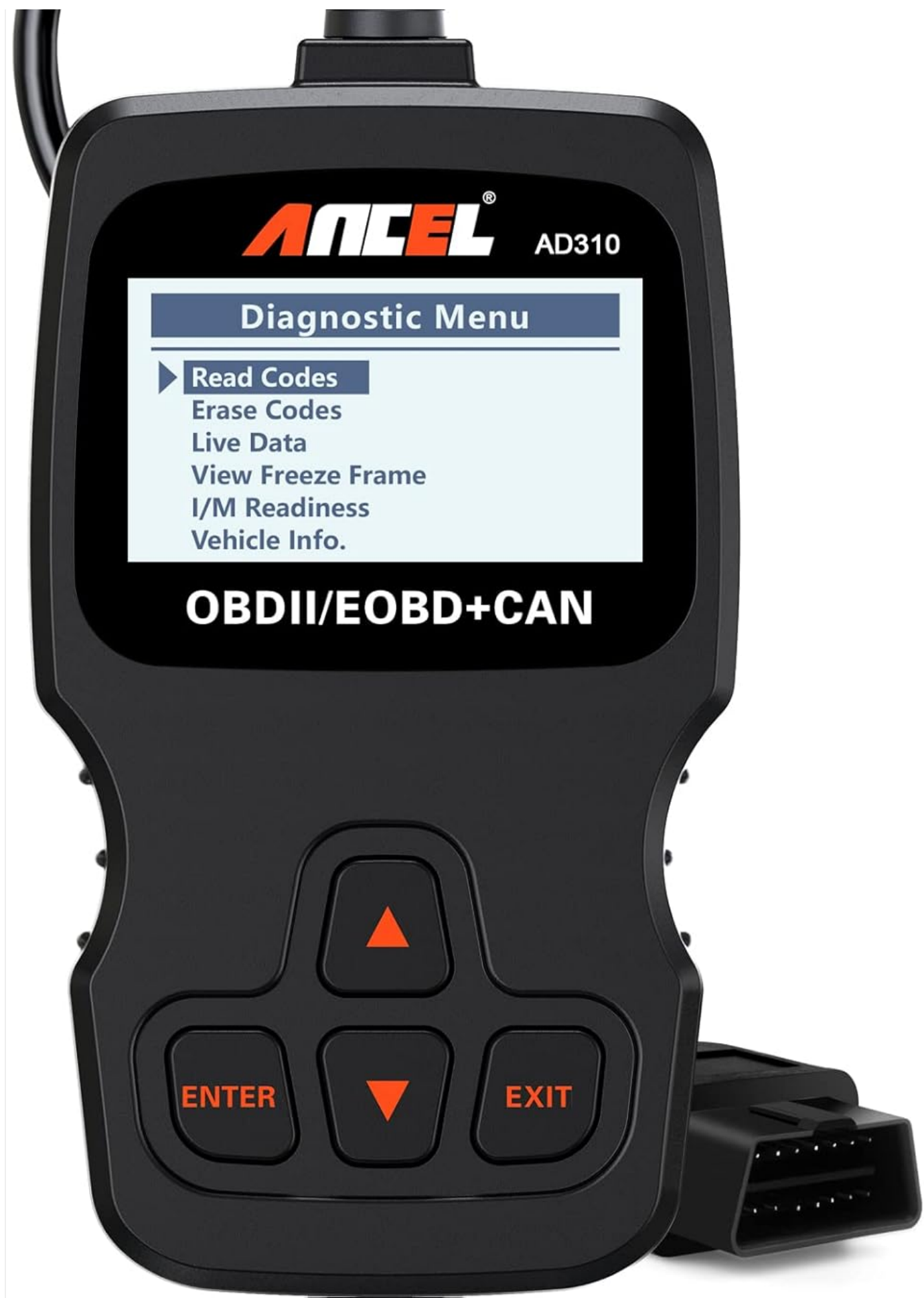
Image: The ANCEL AD310's monochrome screen displaying the "Diagnostic Menu" with options like Read Codes, Erase Codes, Live Data, and I/M Readiness.
