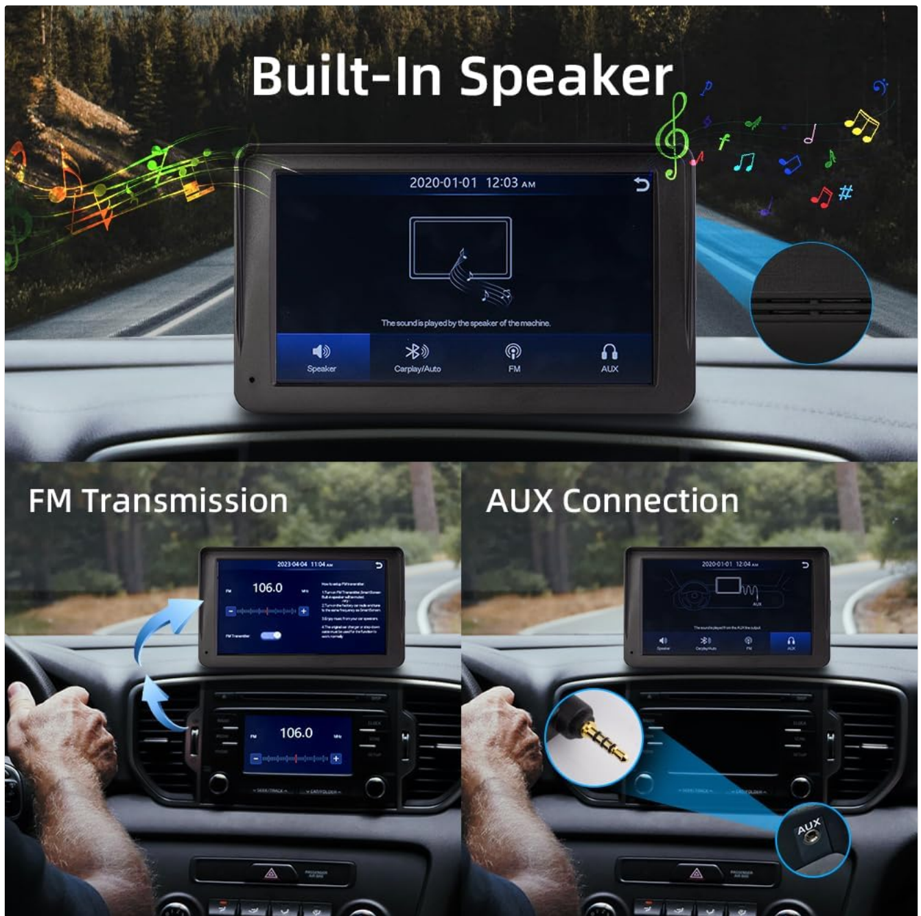
Figure 16: Overview of audio output options: built-in speaker, FM transmission to car radio, and direct AUX cable connection.
