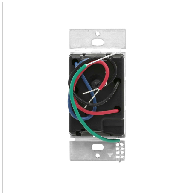
Image: Rear view of the Lutron Caseta Smart Claro Accessory Switch, showing the various colored wires for connection (green for ground, black for common, red and blue for travelers).
