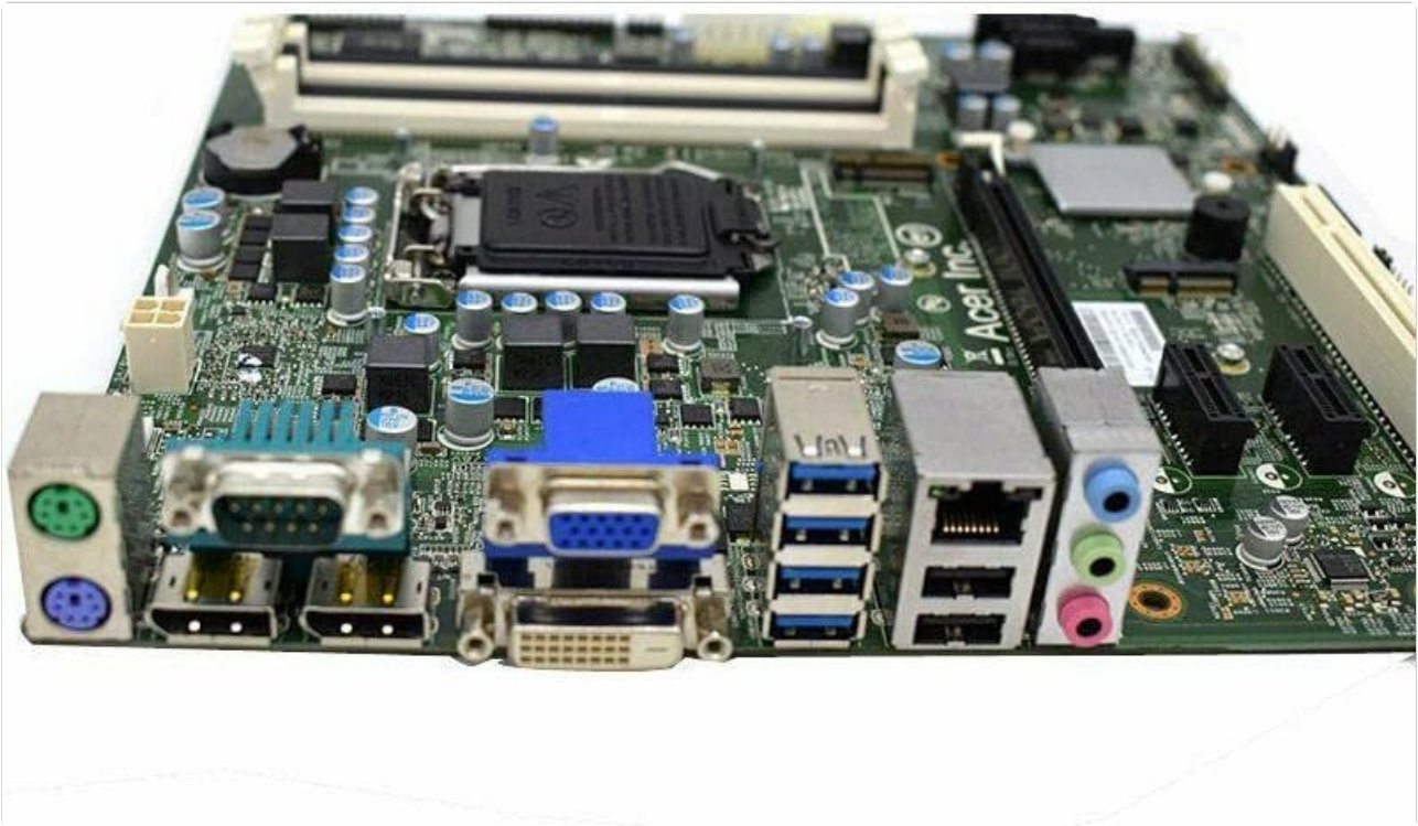
Figure 2: Rear Input/Output (I/O) Panel. This image displays the array of external ports available on the motherboard, including multiple USB ports, video outputs (HDMI, VGA), an Ethernet port, and audio jacks for connecting peripherals.
