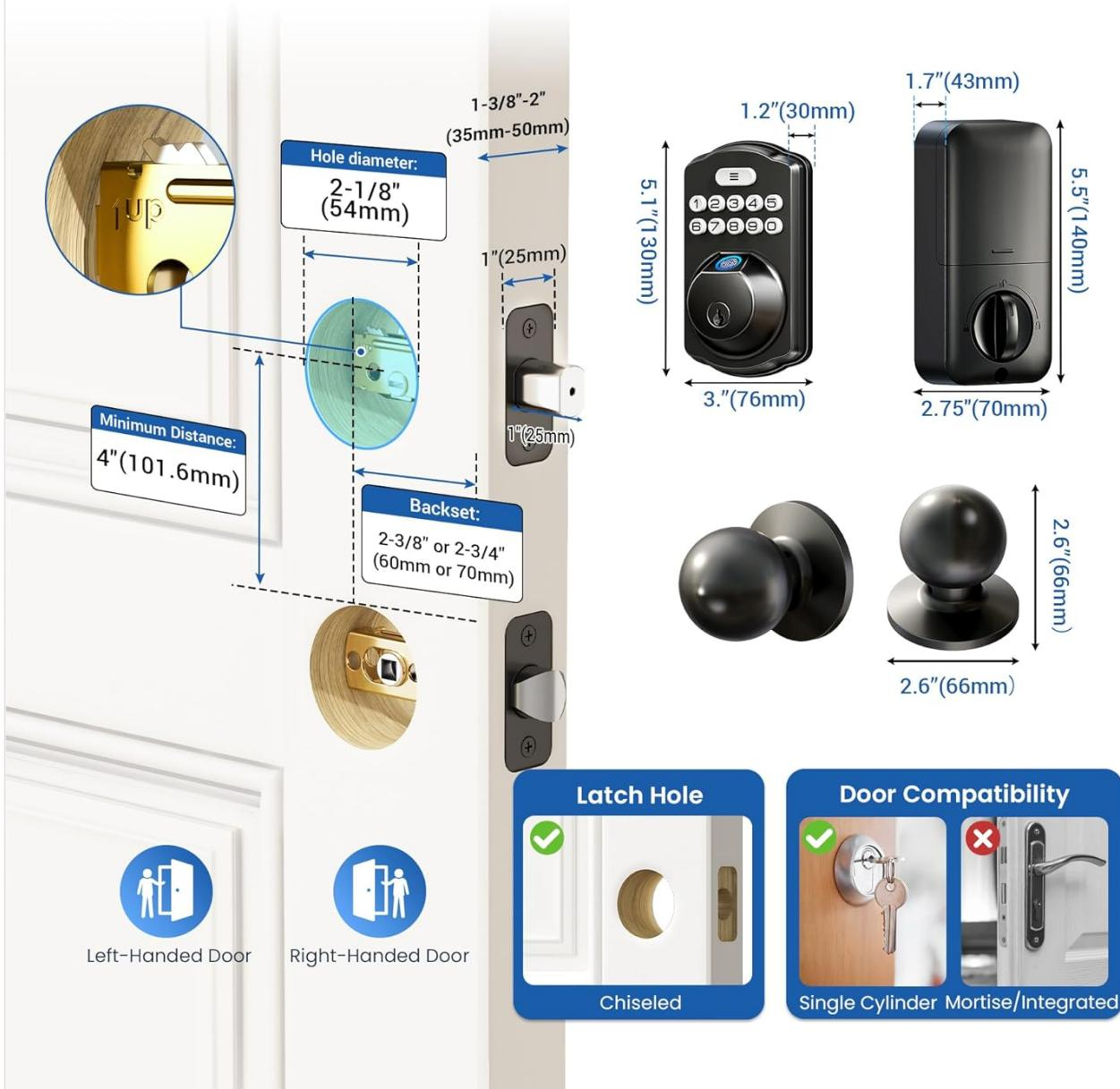
This diagram illustrates the necessary door dimensions and compatible lock types for installing the Veise KS02C Fingerprint Door Lock. It shows hole diameters, backset measurements, and acceptable latch hole designs.
