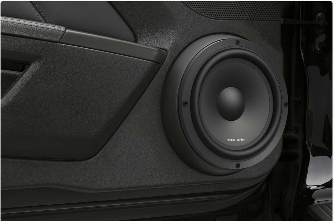
Figure 4.1: Woofer installed in a vehicle door panel.
