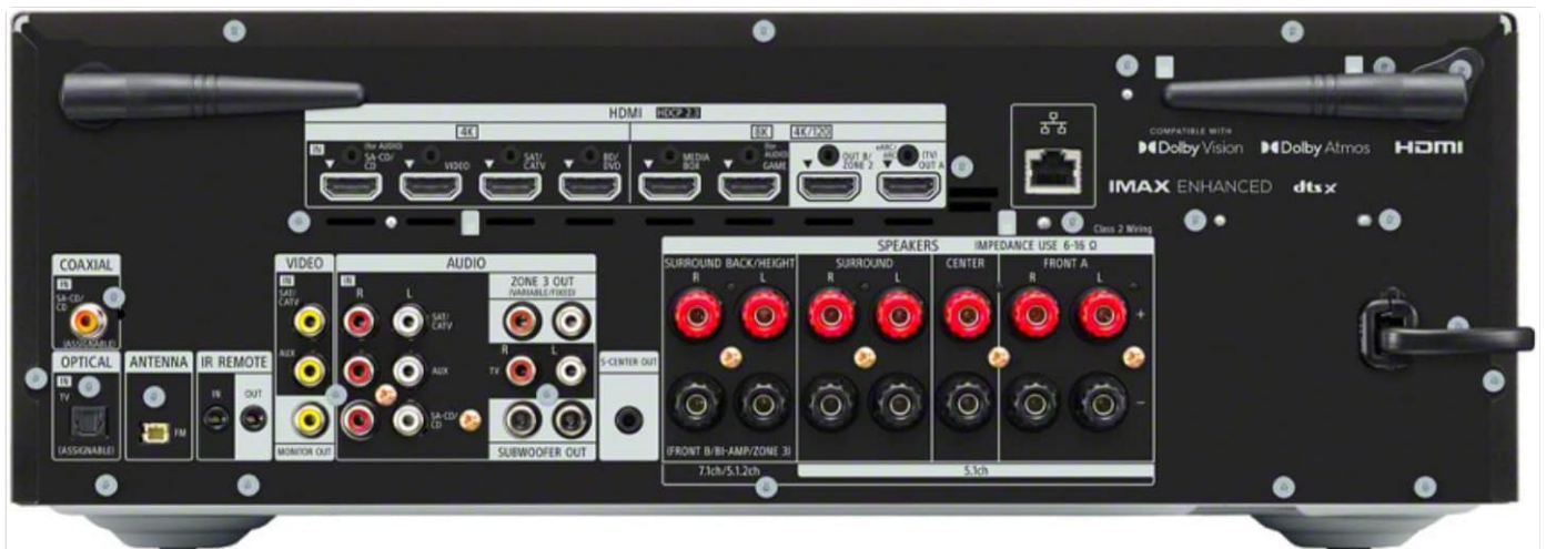
Figure 4: The rear panel of the STR-AN1000 receiver, displaying the comprehensive array of HDMI, audio, and speaker terminals. This view is crucial for understanding connection points.
