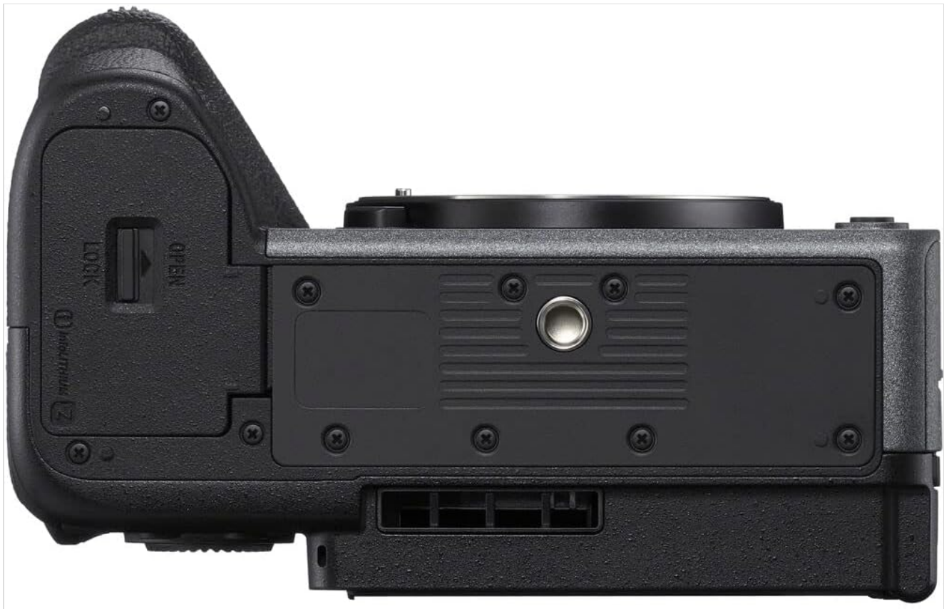
Figure 4.6: Left side view of the Sony FX3, revealing the battery compartment and dual CFexpress Type A/SDXC card slots, secured by a lock/open mechanism.
