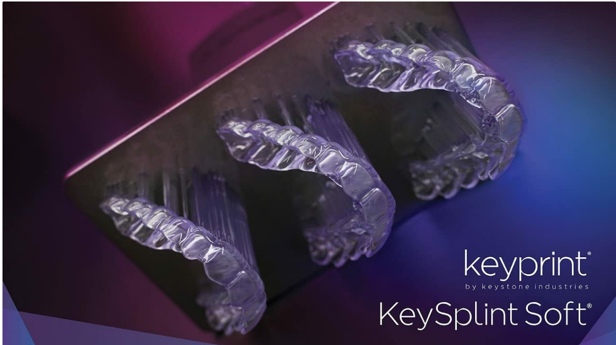
Image 3.1: KeySplint Soft dental splints being printed on a 3D printer build plate.
