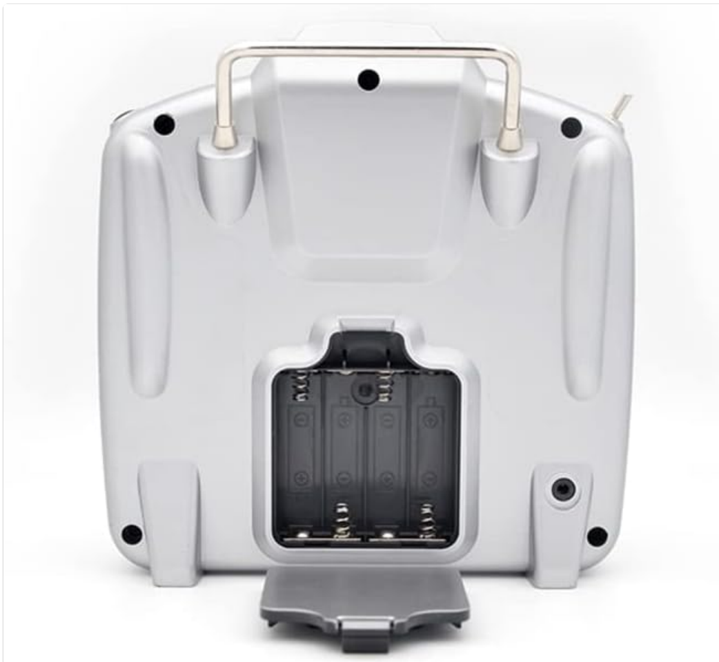
Figure 4.1: Rear view of the MC6C transmitter with the battery compartment open, showing the slots for four AA batteries.
