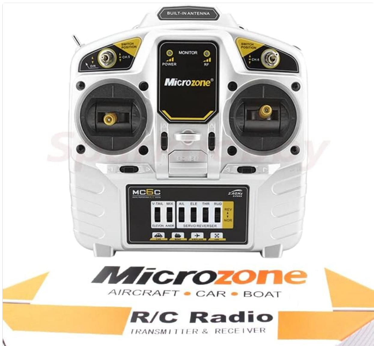
Figure 2.2: Front view of the MicroZone MC6C transmitter, showing the gimbal, switches, and display panel.
