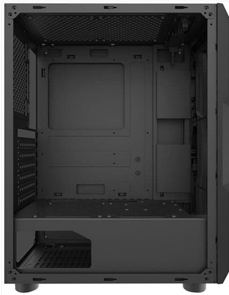
Figure 3: Interior view of the darkFlash Aquarius Mesh case, highlighting the motherboard tray and cable routing options.
