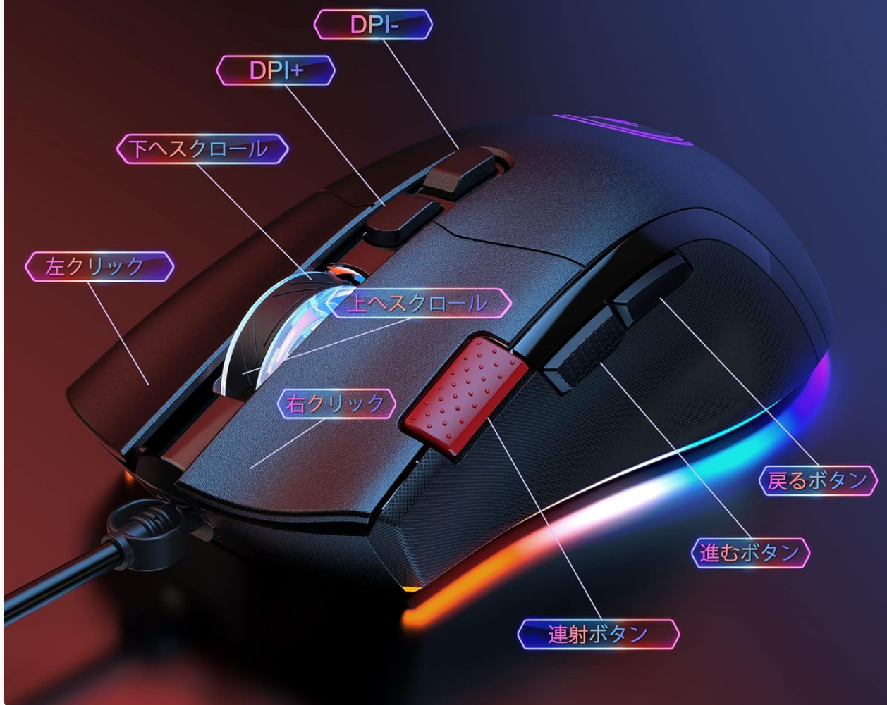
Image 3.1: Layout of the 9 programmable buttons on the GM003-1 mouse.
