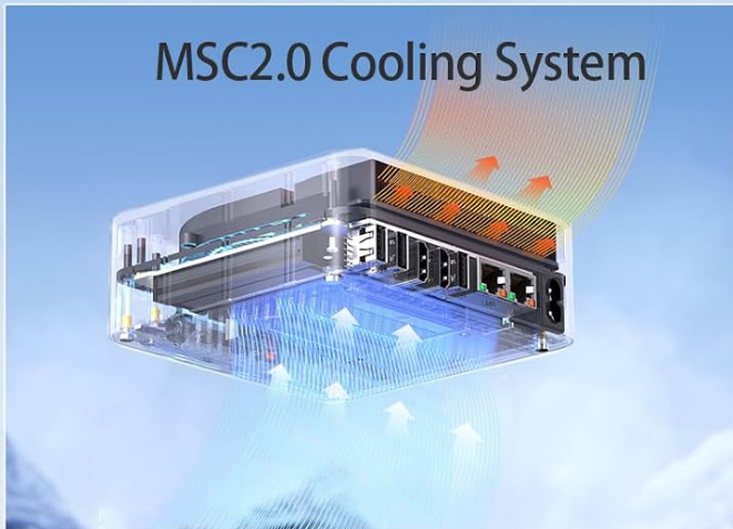
Figure 6: Internal design highlighting MSC2.0 cooling system and dustproof features
