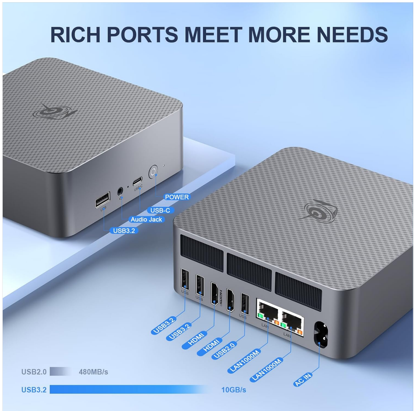
Figure 2: Rear and Front Ports of Beelink EQR6 Mini PC
