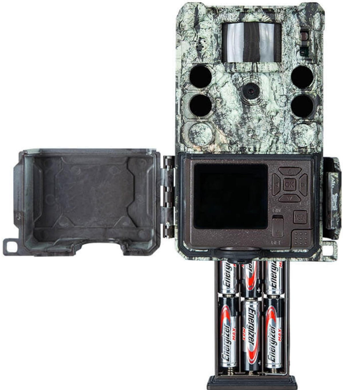
Figure 3.1: Battery tray removed for battery installation.
