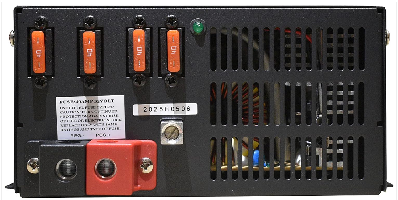
Image: Rear view of the charger, highlighting the fuse panel and battery connection terminals.
