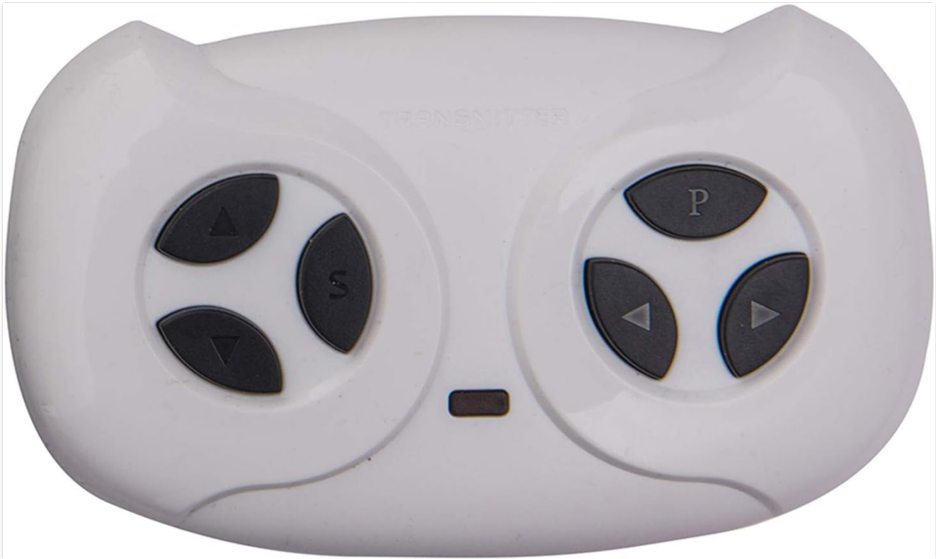
Image: A clear view of the JR1922RXS-2 remote control, showing the button layout. The left joystick-like buttons control movement, and the right buttons control speed and braking.
