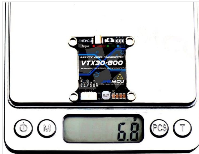
Image: The VTX30-800 module being weighed on a digital scale, indicating a weight of 6.8 grams.
