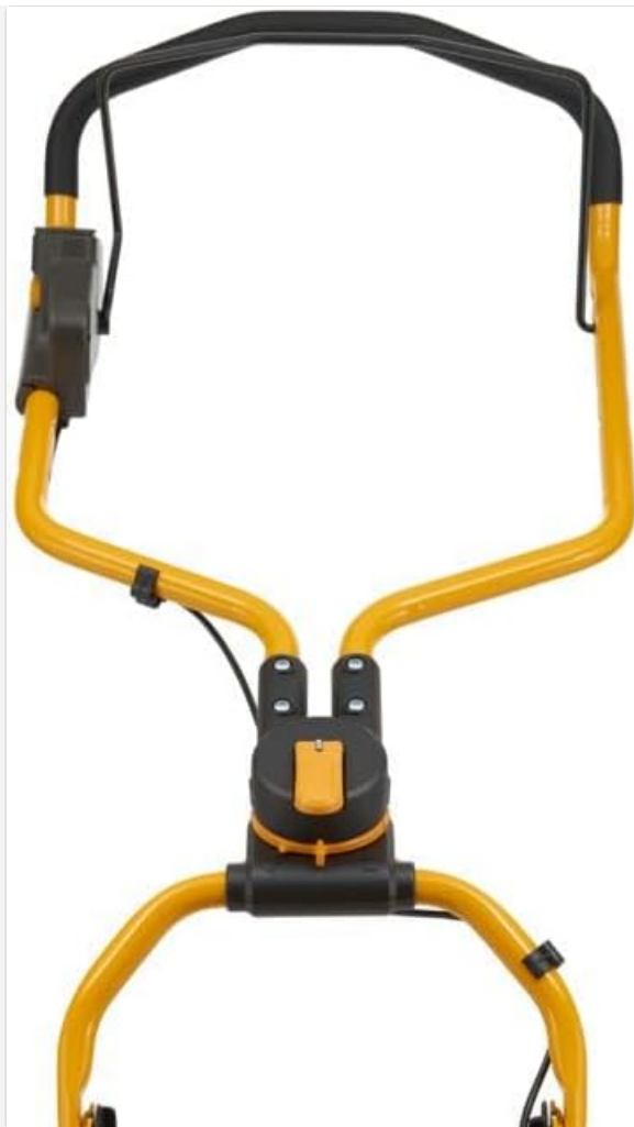
Figure 4.1: Top view of the handle, showing the safety button and bail lever for starting the mower.
