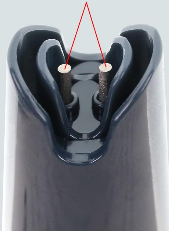
Figure 2: Close-up view of the durable titanium alloy sensor for conductivity measurements.
