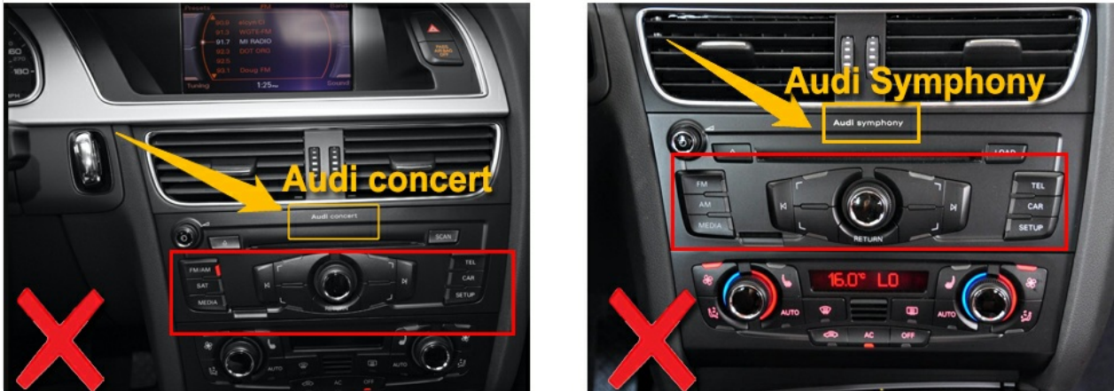
Image 2.2: Examples of Audi Concert and Audi Symphony systems, which are not compatible.
