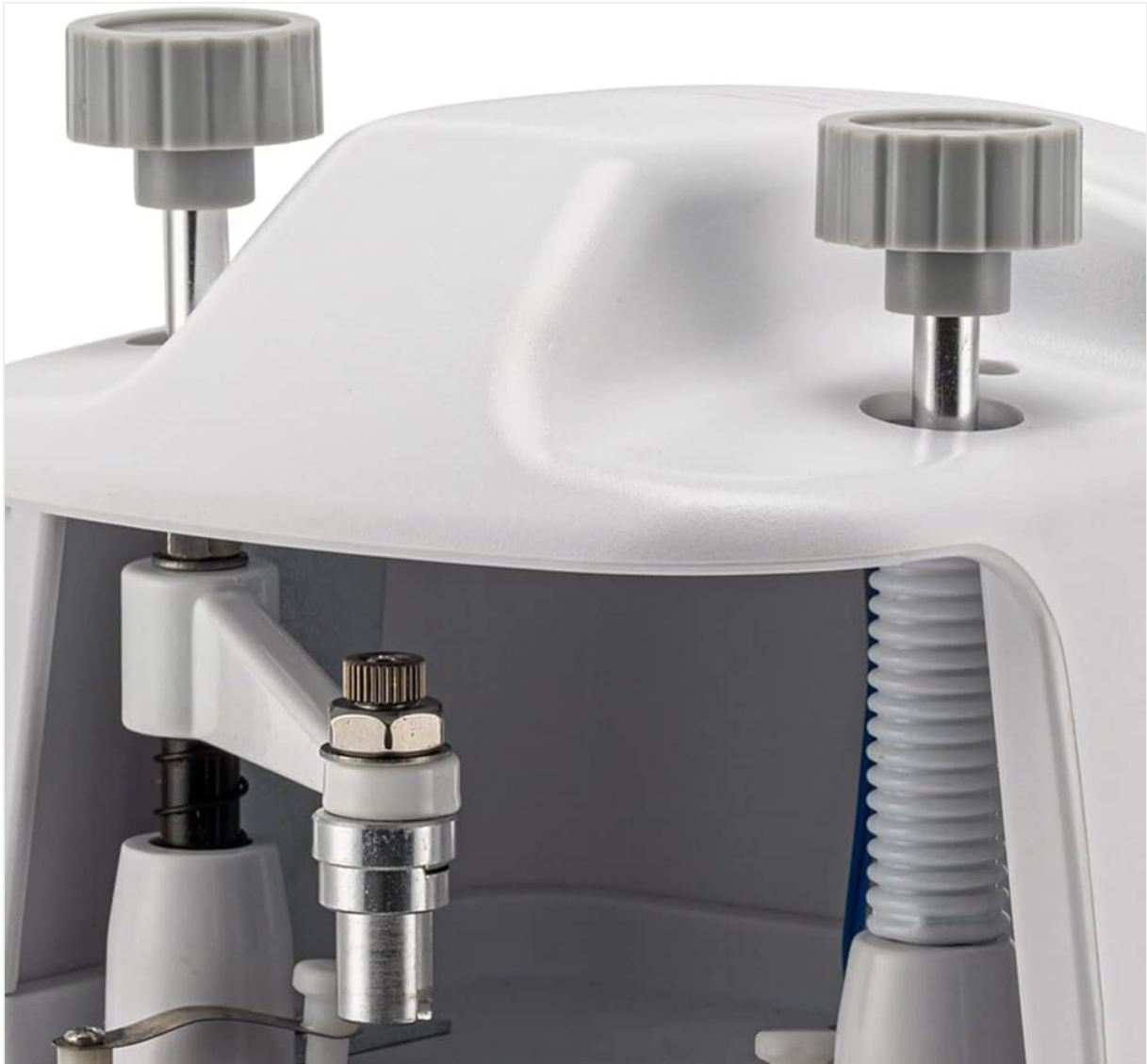
Figure 5.2: Top view of the device, highlighting the two main control knobs used for adjustments during the centering process.
