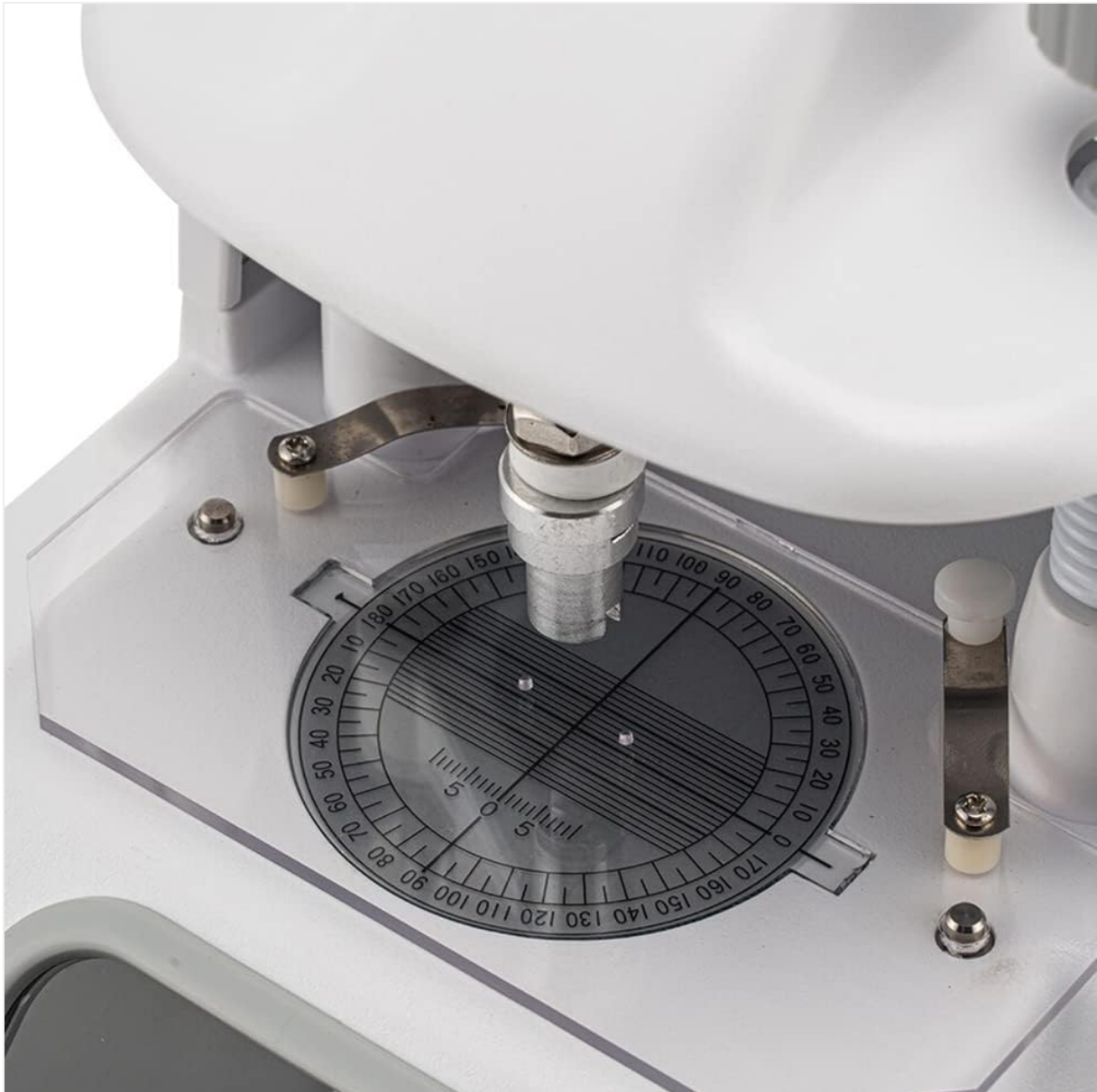
Figure 5.1: Detailed view of the measurement platform, showing the circular guide for lens placement and the central alignment point.
