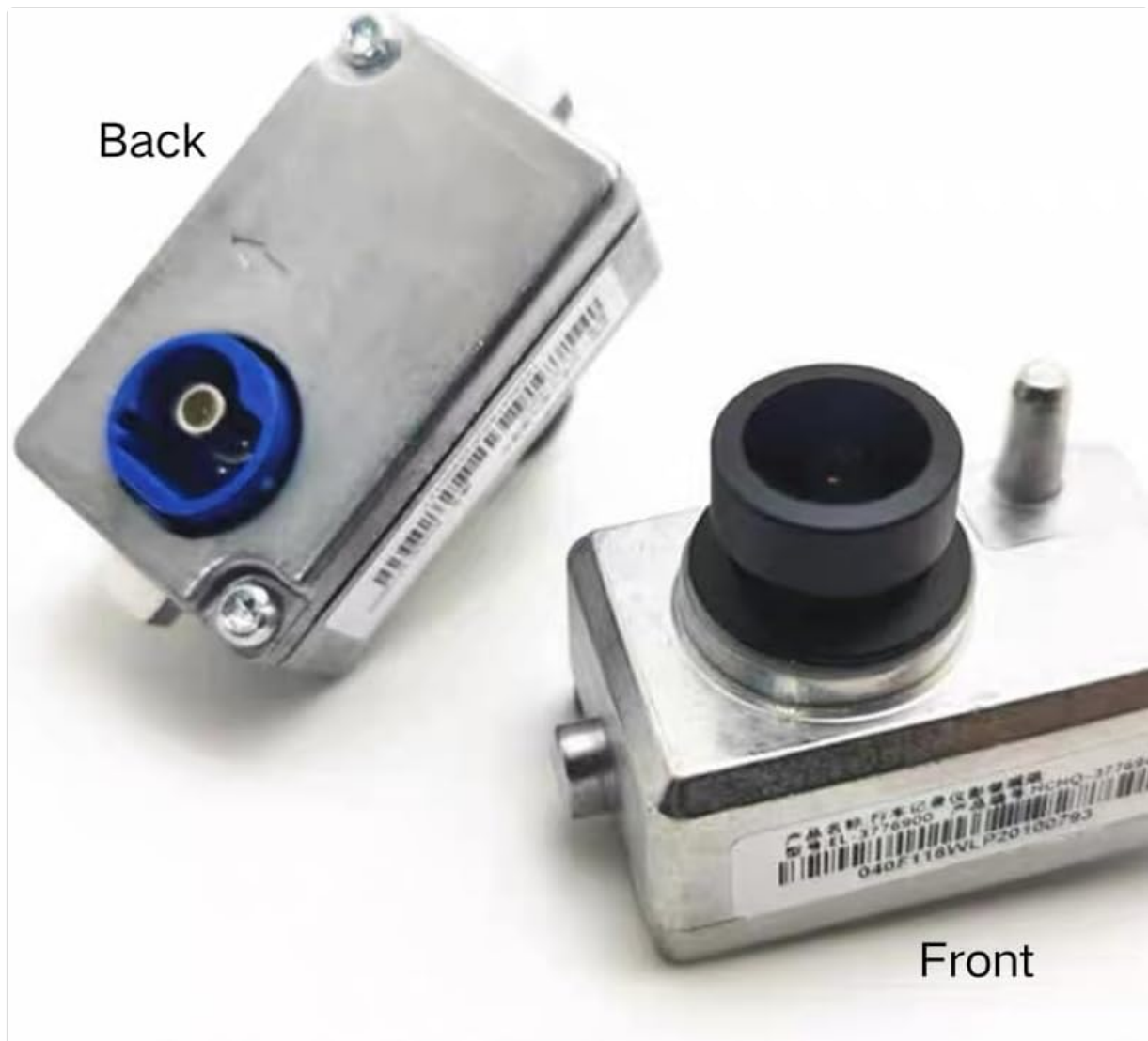
Image 2.1: Front and back view of the dash cam unit. The front features the camera lens, while the back shows the blue connector port.
