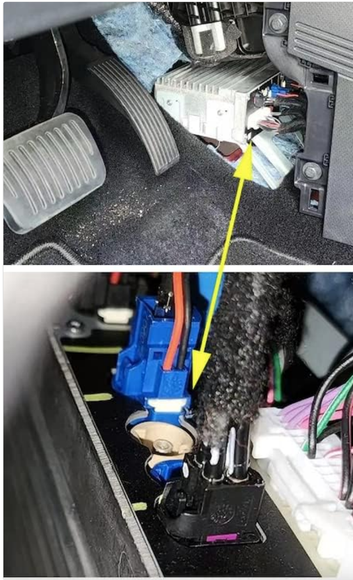
Image 3.1: Illustration of the blue connector port on the vehicle's main unit, indicated by a yellow circle and arrow. This is where the dash cam connects.
