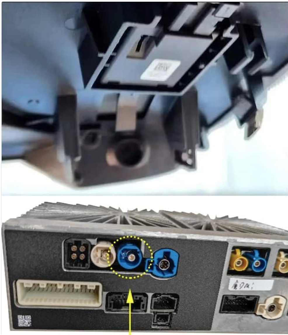
Image 3.3: A close-up view of the connection point for the dash cam, showing the blue connector.
