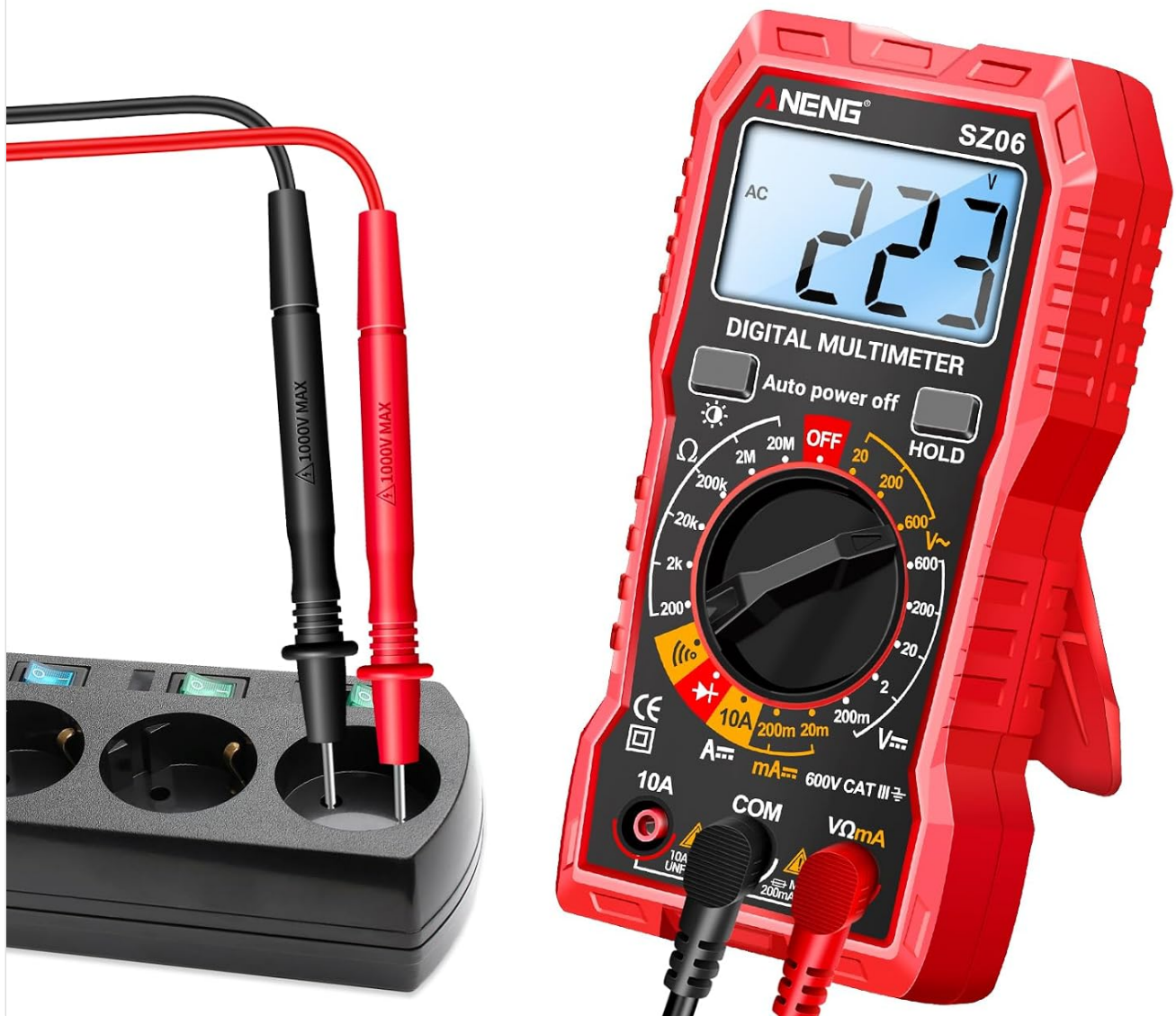
Figure 4.1: Measuring AC voltage using the multimeter.
