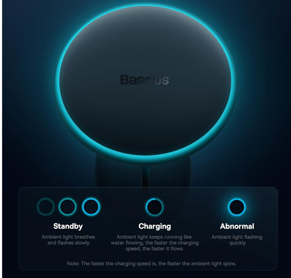
Figure 6: Ambient Light Ring indicating different statuses.
