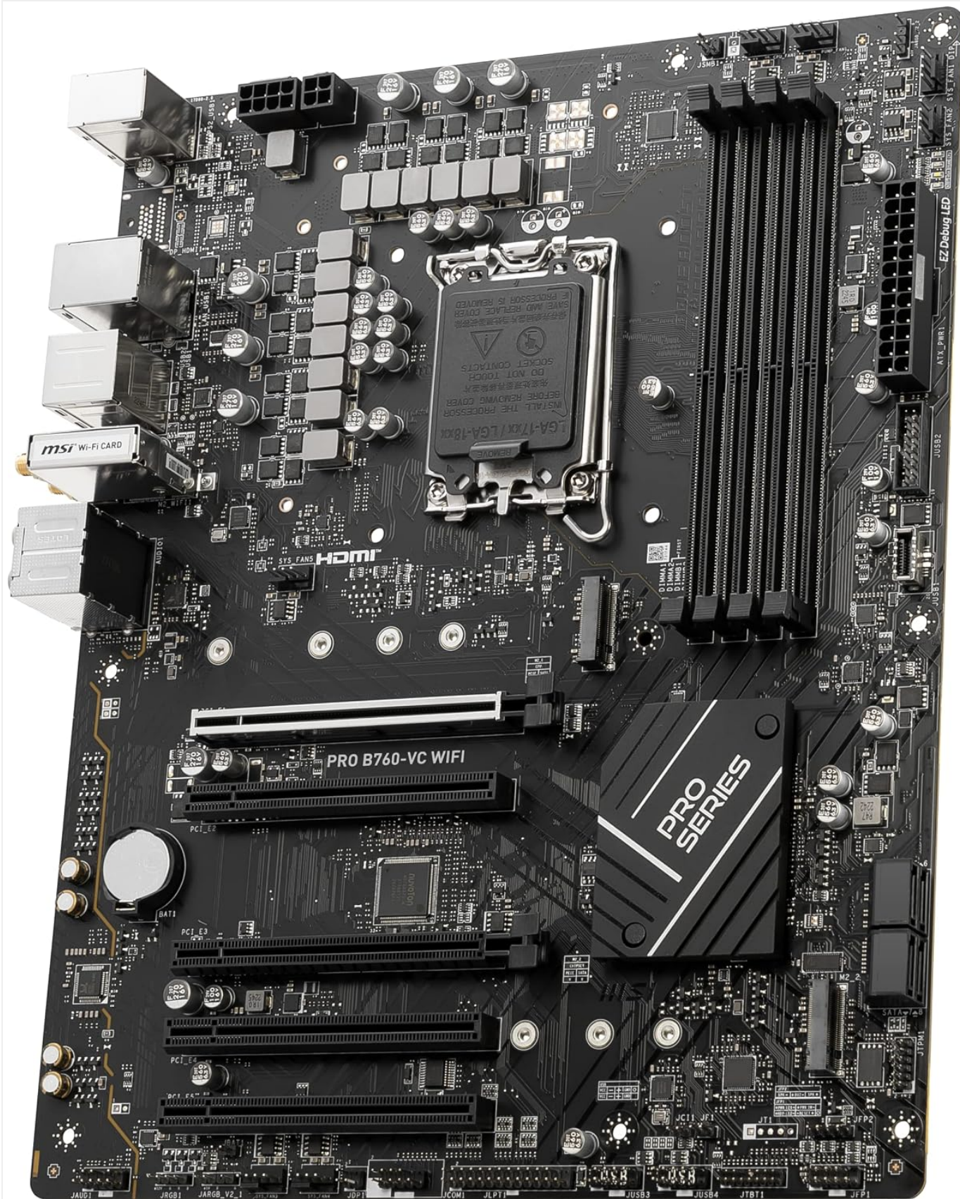
Image: Angled view of the MSI PRO B760-VC WiFi motherboard, highlighting the rear I/O panel and power delivery components.
