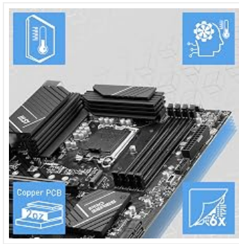
Image: Graphic illustrating the integrated cooling features and the 6-layer PCB with 2oz copper.
