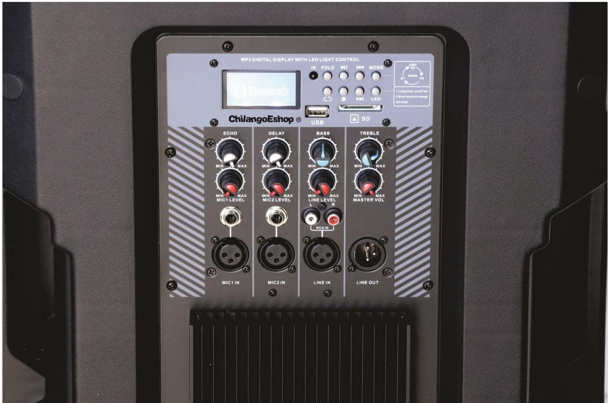
Figure 4.3: Control Panel. A detailed view of the control panel, featuring an MP3 digital display, Bluetooth connectivity indicator, USB and SD card slots, various input ports (XLR, 6.3mm Jack, RCA), and control knobs for Echo, Delay, Bass, Treble, Microphone Levels, Line Level, and Master Volume.
