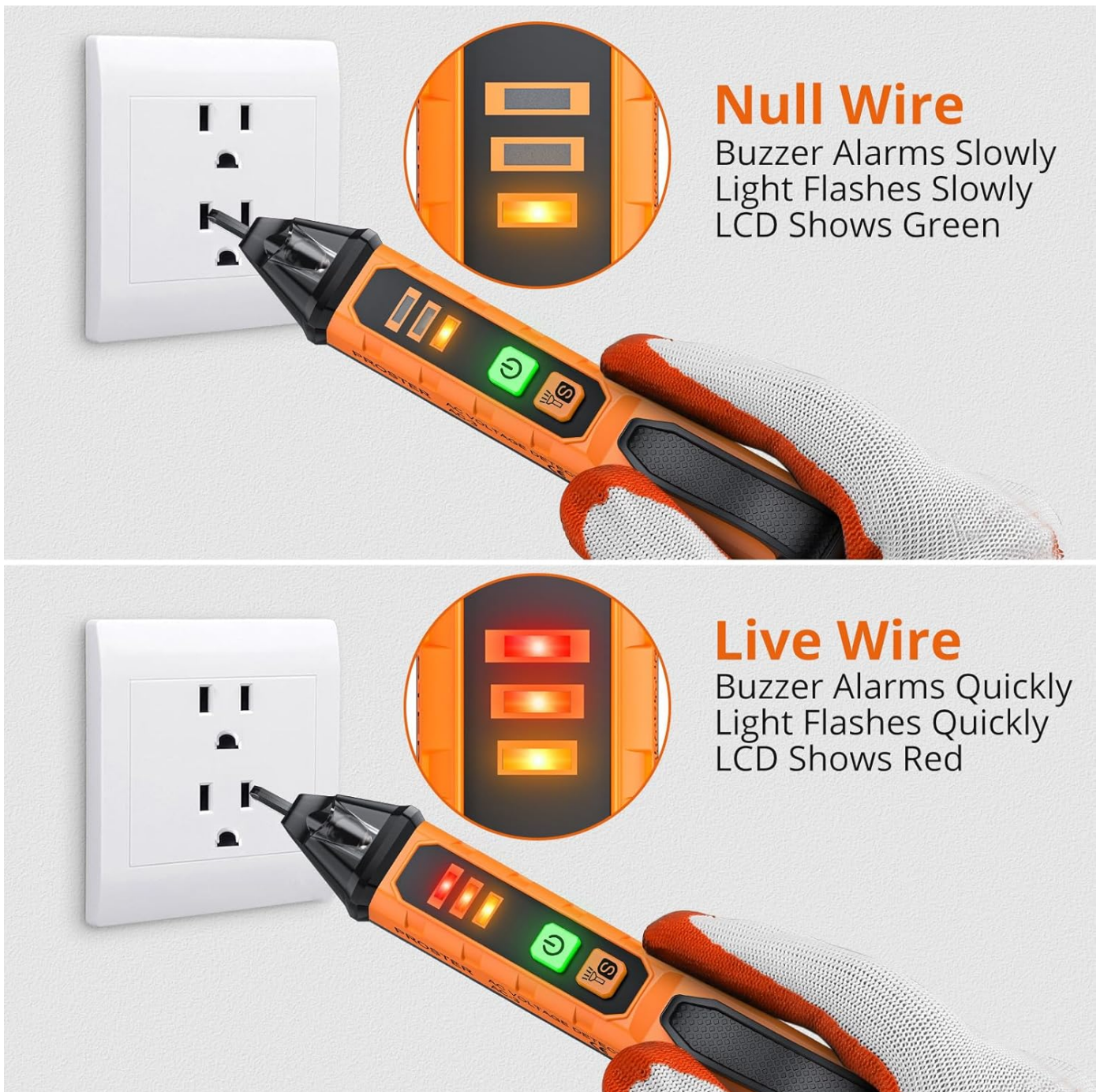
Image 5: Illustration of the tester distinguishing between live and null wires in an electrical outlet.
