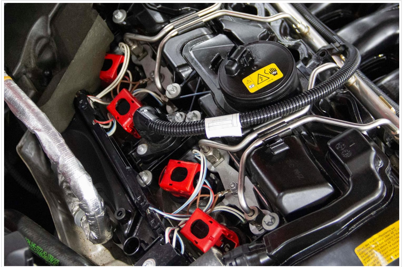
Figure 5: Dinan ignition coils installed in an engine bay, showing their placement relative to other engine components.
