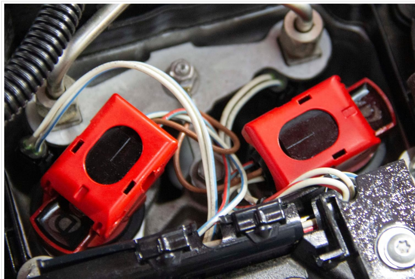
Figure 6: A closer view of two installed Dinan coils, illustrating the connection points and their integration into the engine's ignition system.
