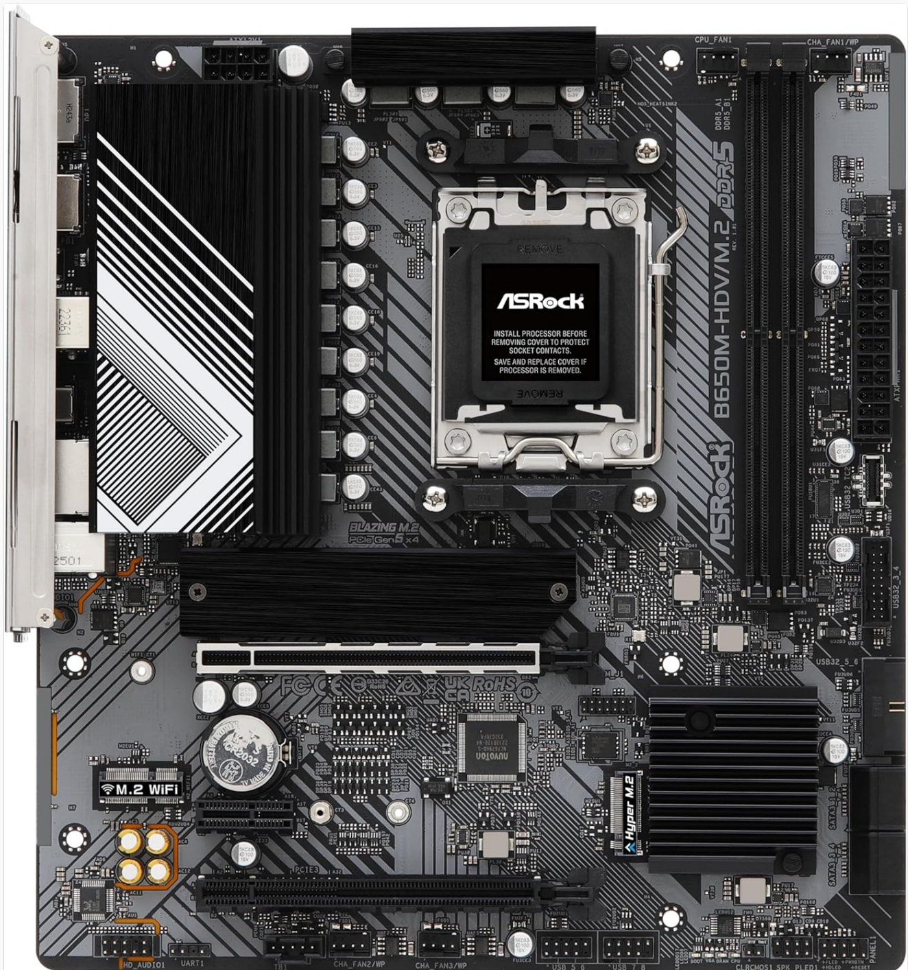
Figure 2.1: Top-down view of the motherboard, highlighting the AM5 CPU socket.
