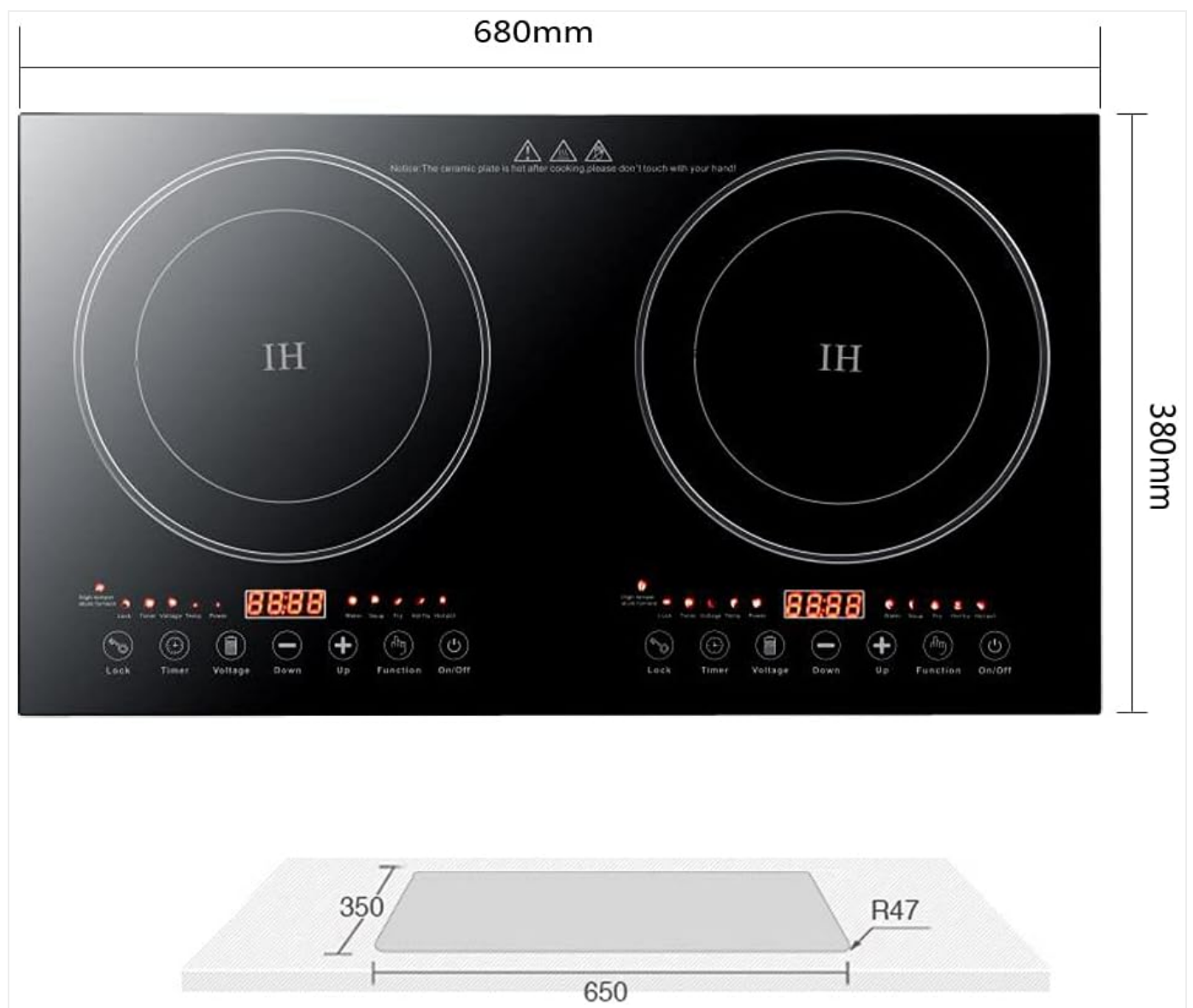
Image: A technical diagram illustrating the dimensions of the induction cooktop, including overall size and recommended installation cutout dimensions.
