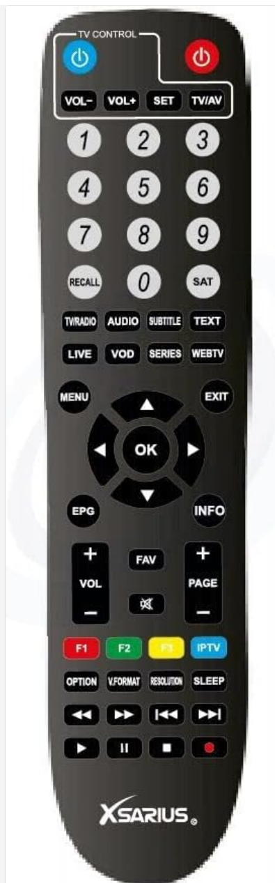
Figure 3.4: The remote control for the Xsarius Sniper X 4K White, featuring various control buttons for navigation, media playback, and specific functions like Live TV, VOD, and EPG.
