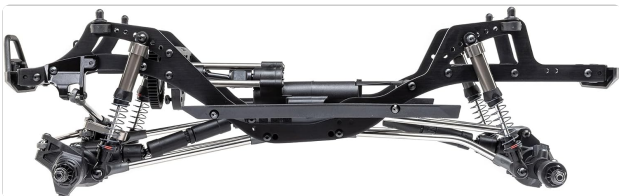
Side view of the assembled Axial SCX10 PRO chassis, showing the suspension and drivetrain.
