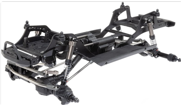
Assembled Axial SCX10 PRO chassis from a front-left perspective.
