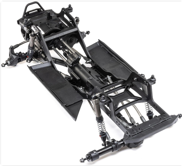
Assembled Axial SCX10 PRO chassis from a top-down perspective.
