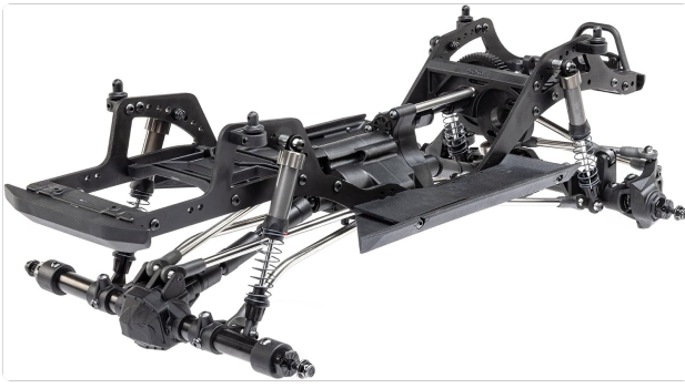
Assembled Axial SCX10 PRO chassis from a rear-right perspective.
