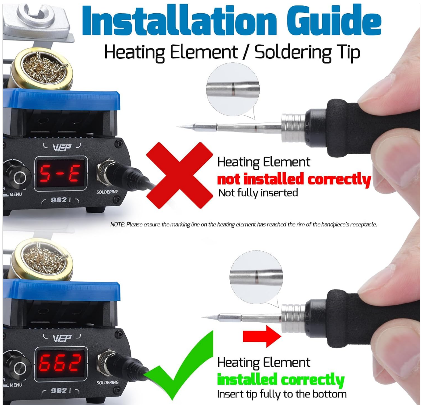
Figure 4: Incorrect tip installation (not fully inserted).
