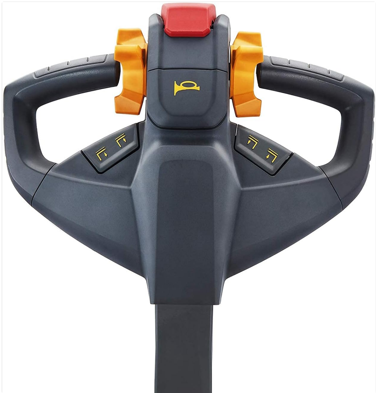
Figure 2: Close-up of the ergonomic control handle, illustrating its design and button layout.
