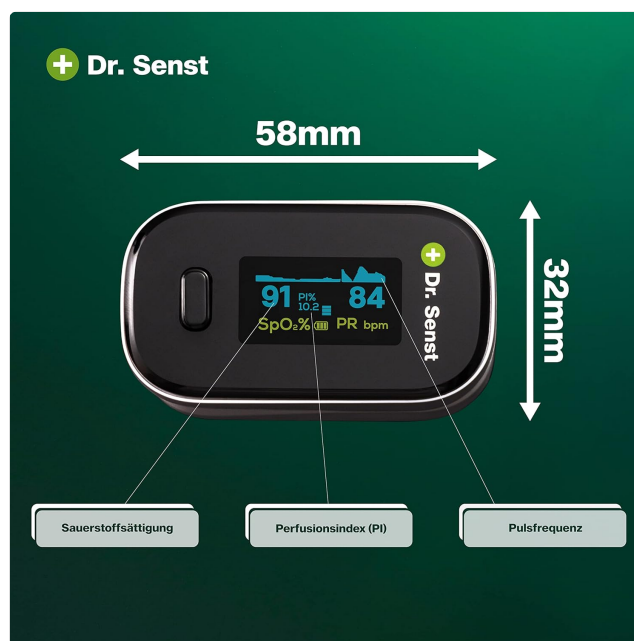
Figure 3: Display elements and dimensions of the Dr. Senst Pulsoximeter YK-80B. This image shows the device's compact size (58mm x 32mm) and points out the Oxygen Saturation (SpO2), Perfusion Index (PI), and Pulse Rate (PR) indicators on the display.
