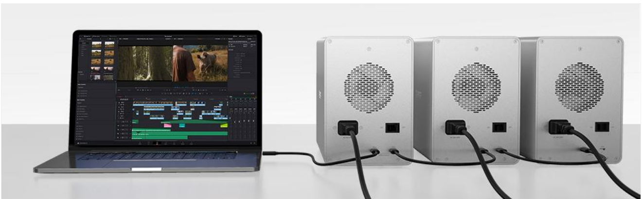
Figure 4.2: Illustrative diagram of daisy-chain connection for storage expansion.
