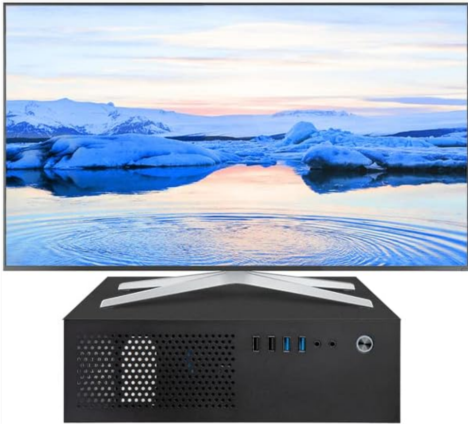
Figure 2.2: Front panel of the JOYJOM MATX Case displaying USB ports, audio jacks, and power button.
