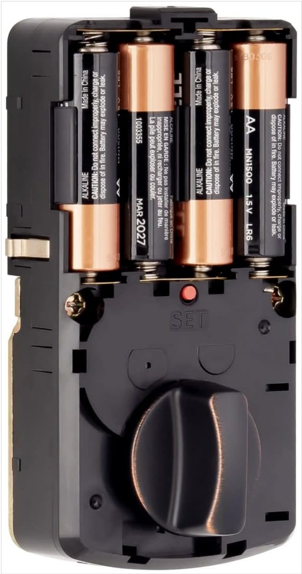
Figure 3.1: Interior unit with battery cover removed, showing the battery compartment and the 'SET' button for programming.
